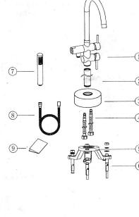
1.Connect the straight tube, decorative tube and bolts holder to inlet tube then screw the inlet tube to main body 4. Connect the inlet tube like the drawing bolts
